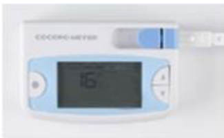
Figure 4.2: Kokorometer to measure salivary amilase level
