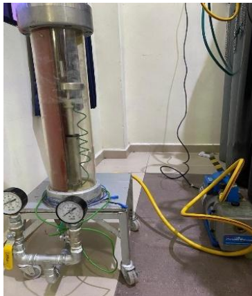
Figure 1.2: Process of removing gas from gas chamber using vacuum pump.
