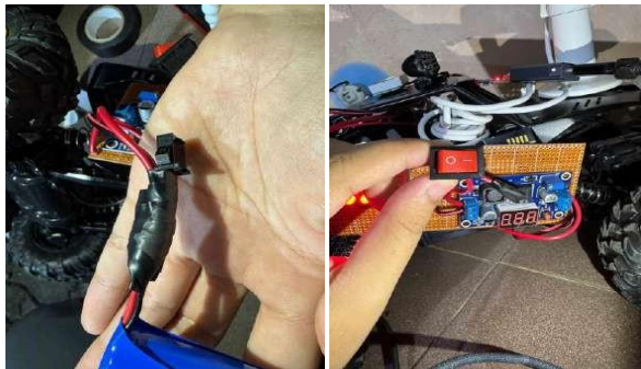
Figure 2.11: Wiring tap assist and switch.
